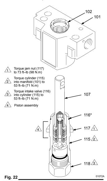
14. Place the ball guide (120), stop pin (122) and ball (121\*) in the cylinder (115). Screw the intake valve into the cylinder and torque to 53 ft-lb (71 N.m). This will also properly torque the cylinder into the manifold. See Fig. 23.
